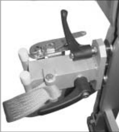
The system is typically used on round masts, including those which differ in diameter over the length of the complete mast.
