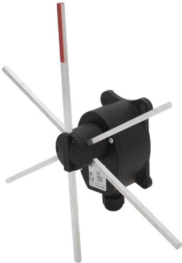
Cross position limit switches designed to control the movement of overhead travelling cranes, hoists and complex machine tools. Tango has rods with maintained positions every 60°.
